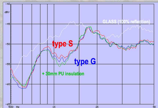
RELATIVE ACOUSTIC ABSORPTION --- MLS ANALYSIS (500-5kHz)
